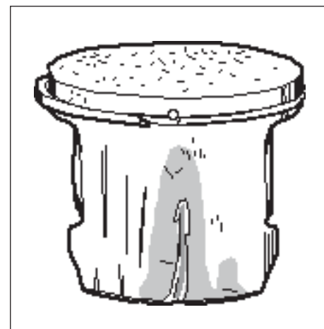
Irregular grooves on the piston's inlet side caused by a broken roller retainer.
