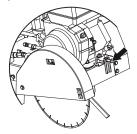
Make sure that the belt pulleys are parallel and aligned with each other. Tighten the screws holding the engine and then unscrew the tension screw 2 turns to prevent it coming into contact with the engine block. Refit the belt guard and tighten the screws holding the belt guard in place.
